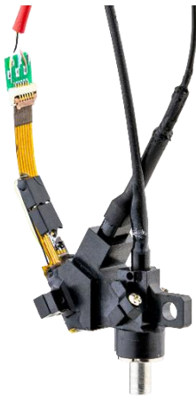
Mini2P microscope with excitation and emission optical fiber and cable harness
