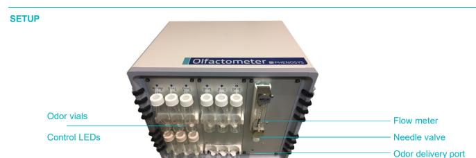
Only Teflon is exposed to the substances downstream of the MFCs. Special valves with low dead volume are used and continuously flushed with neutral gas when not in use with odors. After activation of the odor flow, its concentration equilibrates within 0.5-1 sec.
