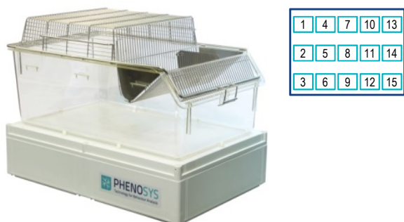
PhenoSys Activity Monitor with 5x3 RFID-reader matrix.
