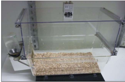
qSIM observation cage with thermal camera and RFID detectors
